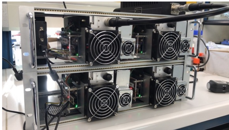
Fig 7.10. PHASESHIFTER Evaluation Kit @ 2.45 GHz.
