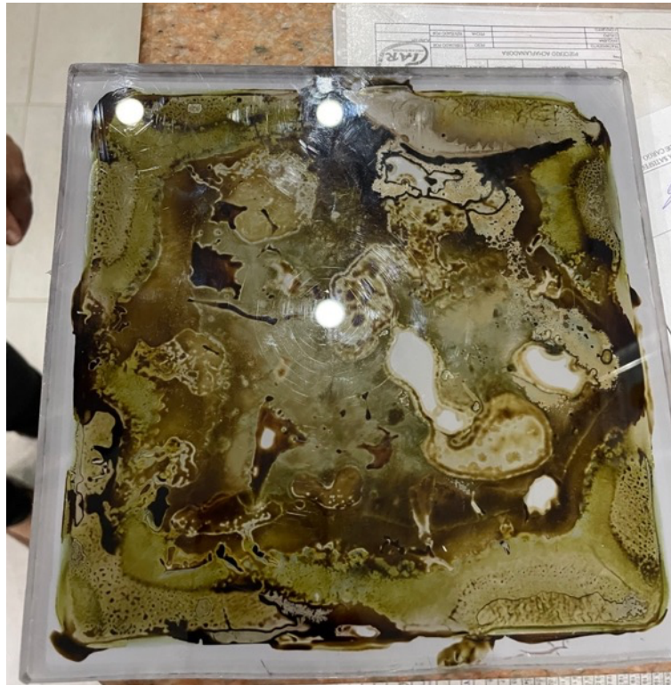
Fig 8.11. Example of the actions performed to verify the proper adhesive distribution.
