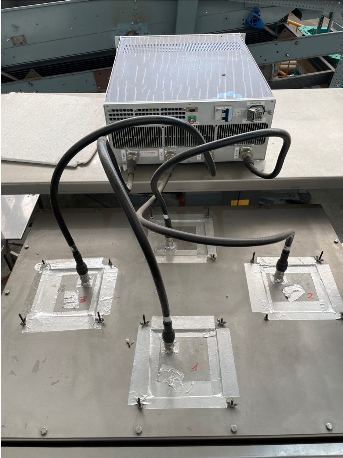
Fig 8.54. Four antennas configuration.
