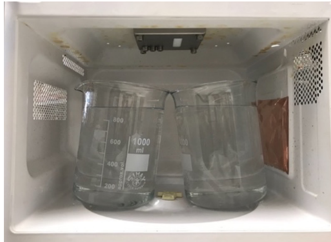
Fig 6.28. 2-litre recipients and the antenna placed in the cavity.
