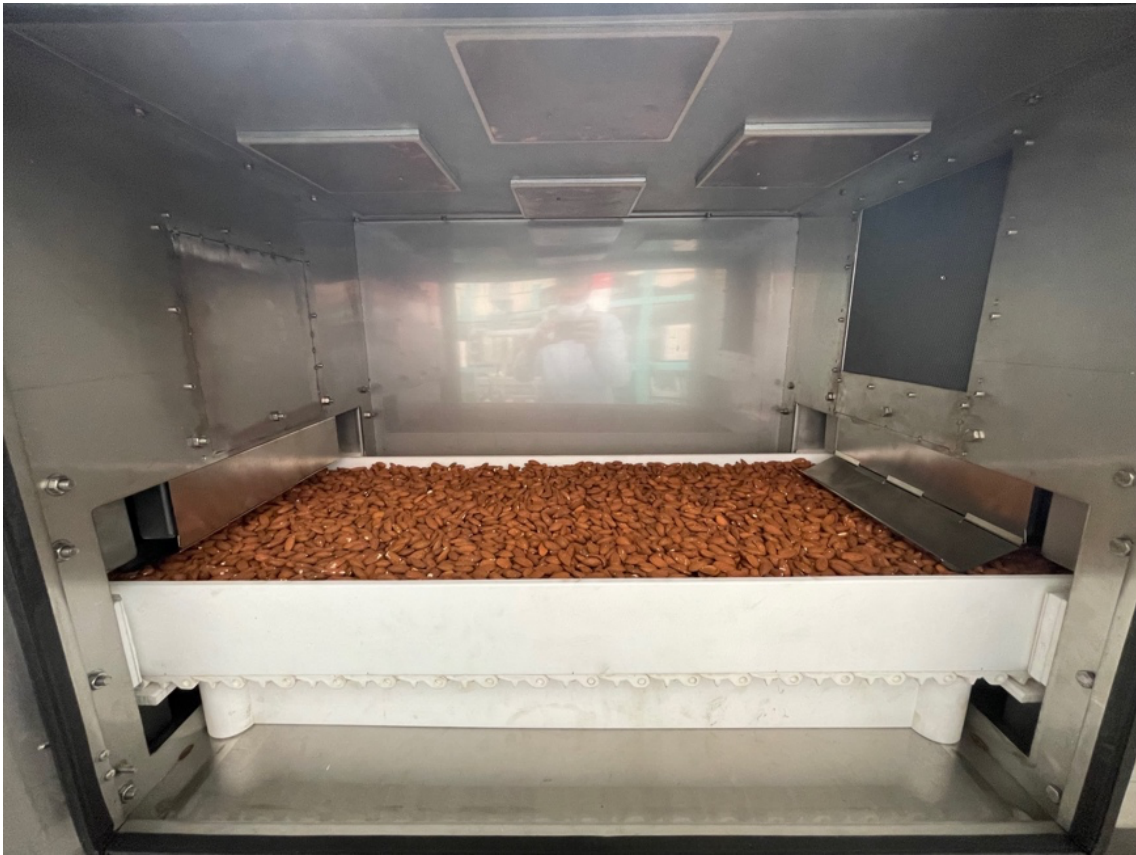
Fig 8.43. Internal view of the transport oven with the almond load and the patch Peek antennas installed on top.
