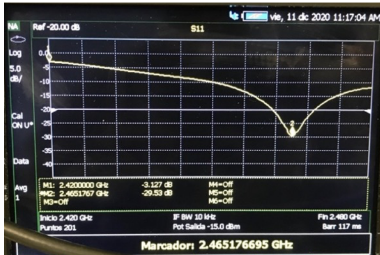
Fig 7.6. Return Losses measurement (S11) of the patch antenna. Marker M2 define the best matching frequency.
