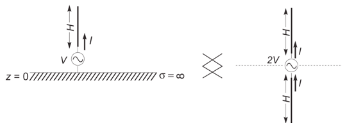
Fig 6.9. Monopole antenna and its equivalent dipole [145, Fig. 4.16]
