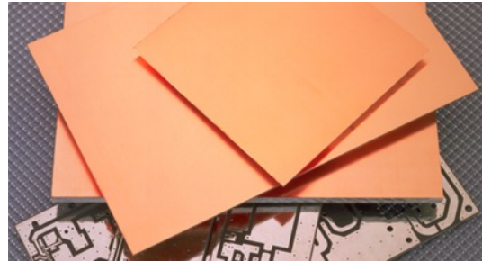
Fig 2.8. RT/Duroid 6202: example of a dielectric used for electronic and microwave circuitry [15]
