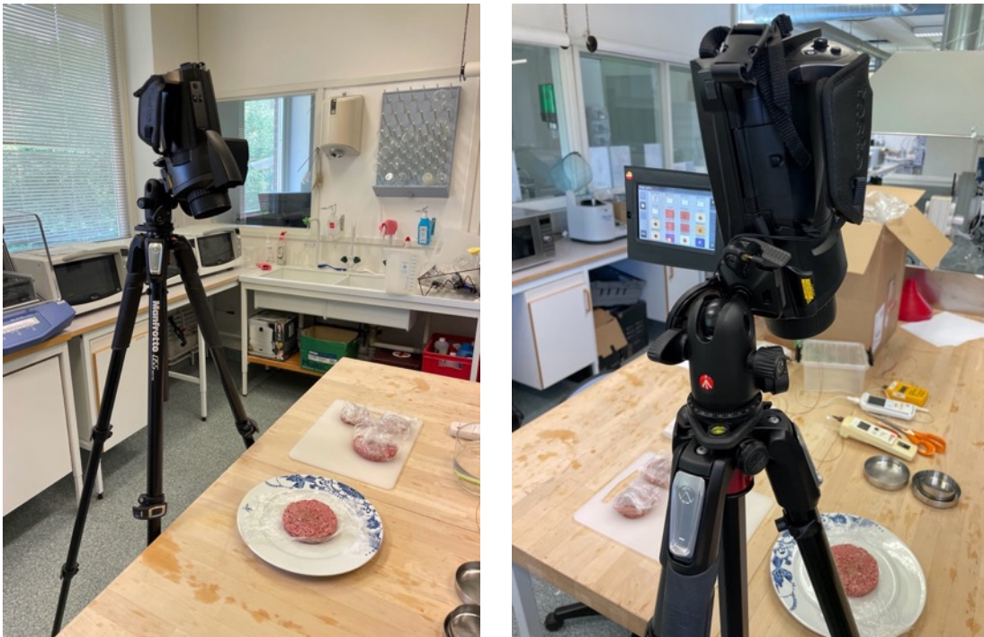
Fig 4.35. Temperature measurement setup at RISE's labs.
