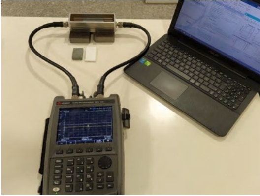
Fig 4.6. Complete measurement system based on CPW probe.
