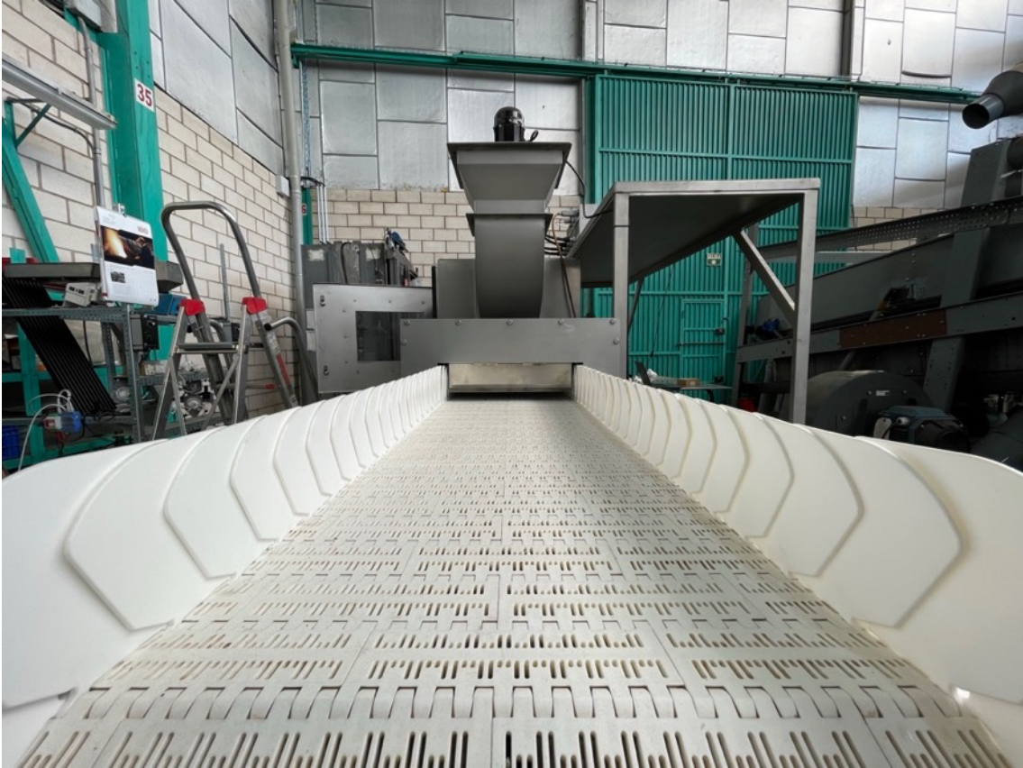
Fig 8.58. Conveyor belt with modular lateral supports to confine the load.
