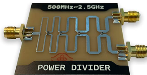
Fig 6.6. Example of a microstrip microwave power divider [141].
