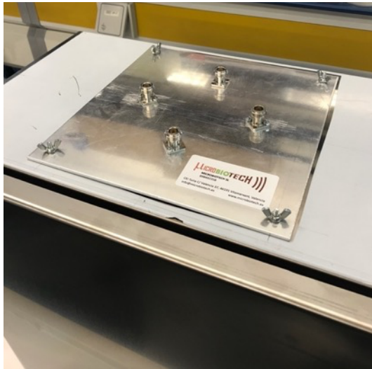
Fig 7.13. Antenna array installed in metallic sheet.
