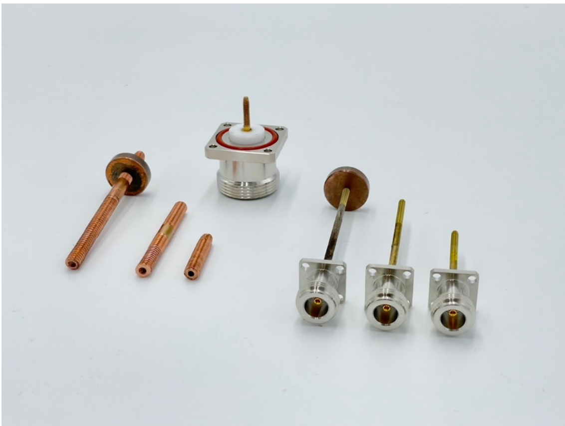
Fig 6.13. Manufactured antennas with the 7/16" connector separately.
