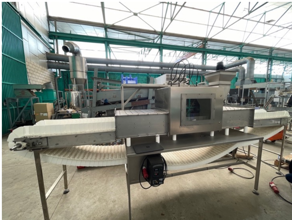
Fig 8.1. Developed conveyor oven for almond drying with the SSMGS at 915 MHz.
