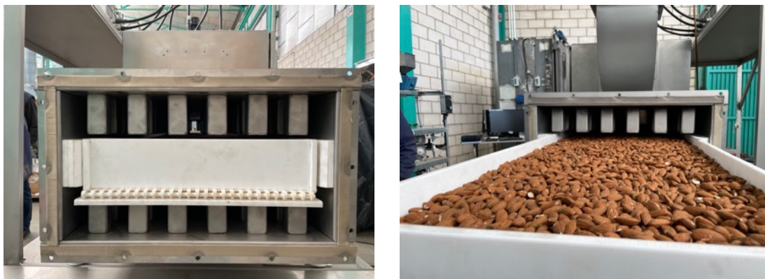
Fig 8.42. Shielding periodic structure installed in the transport oven.
