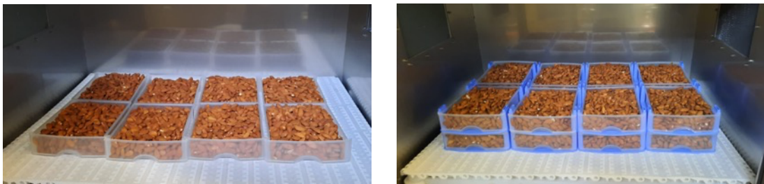
Fig 8.47. Almond distribution with regular compartments for 40 mm (left) and 80 mm (right) thickness.
