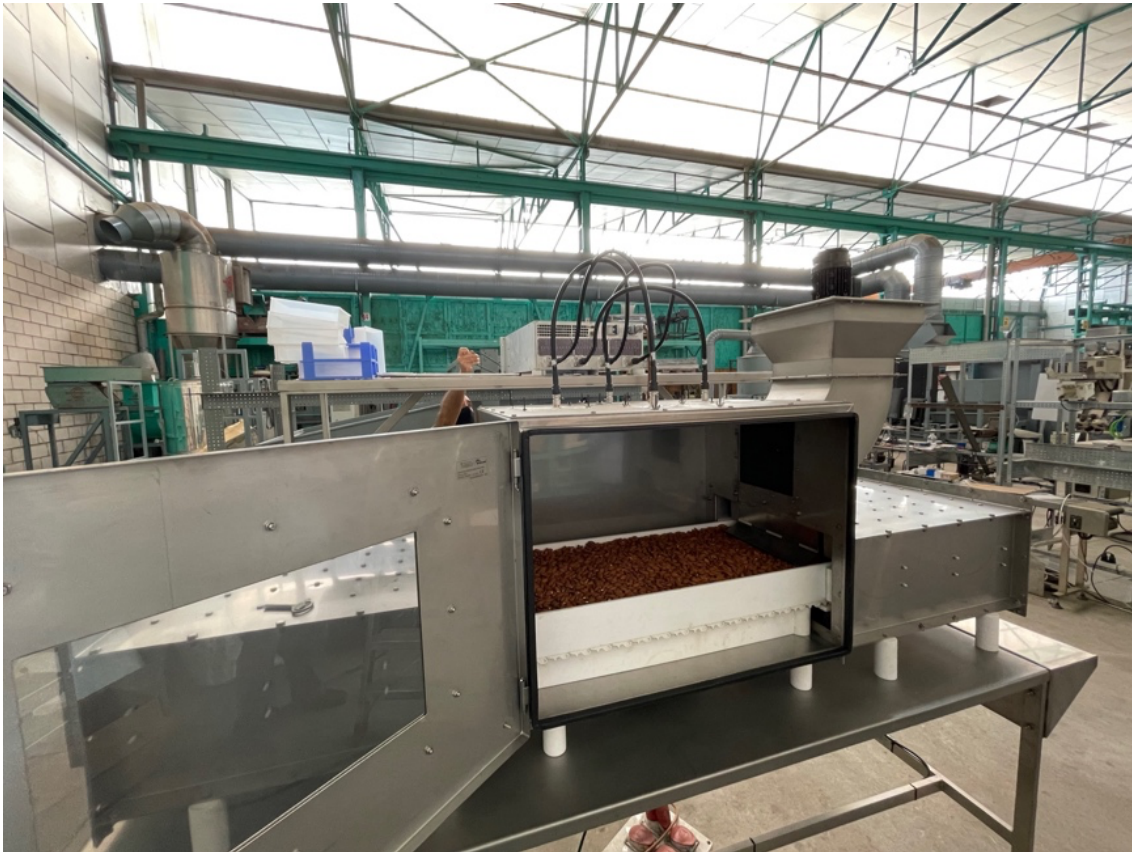
Fig 8.45. External view of the transport oven with the accesses.
