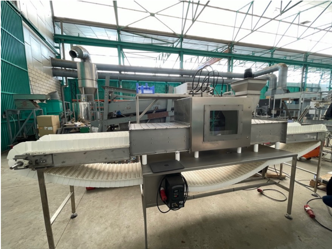
Fig 8.56. Frontal view of the definitive continuous oven with the four sources SSMGS.
