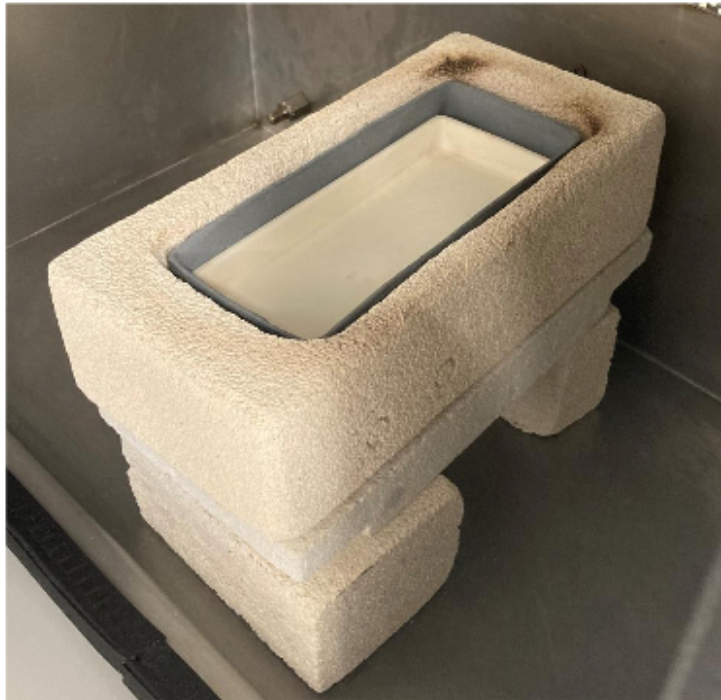
Fig 7.21. Three-layer recipient for microwave-assisted calcination.
