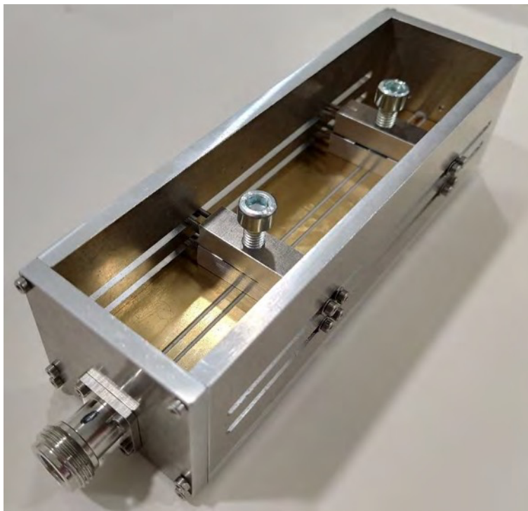
Fig 5.9. Manufactured impedance matching system prototype.
