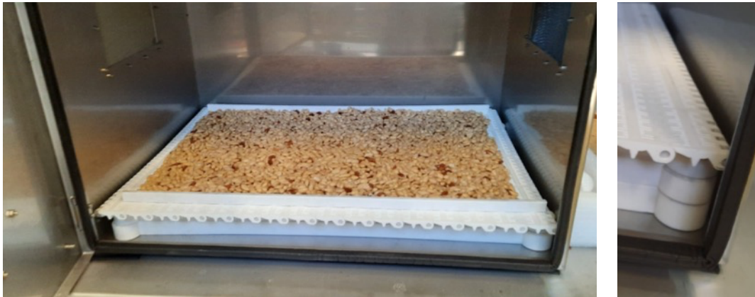
Fig 8.46. Initial load distribution (left) and detail of the elements used to adjust the height of the belt (right).
