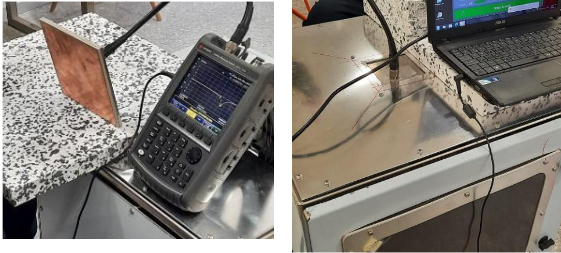
Fig 8.13. Free space measurement with VNA (left) and power tests (right).
