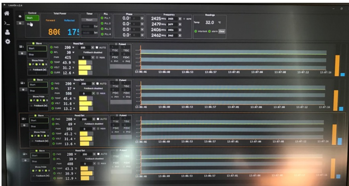
Fig 7.18. Control software screenshot at maximum power where can be seen the Antenna 3 malfunctioning.
