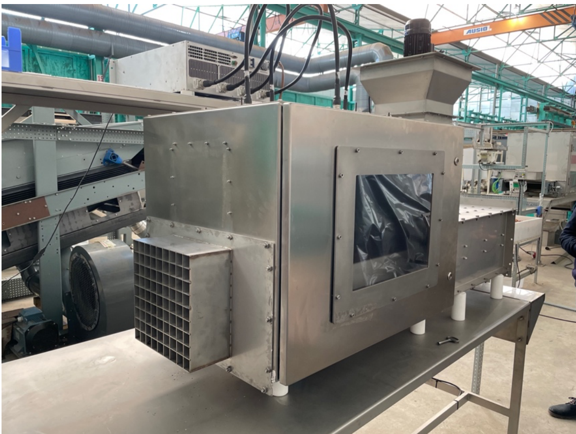
Fig 8.44. Rectangular grid structure that will work as a feed hopper and a shielding element.
