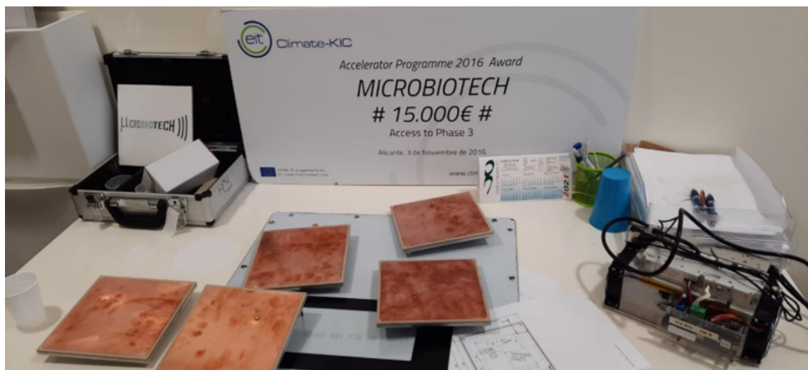
Fig 8.12. Five out of six manufactured antennas and the solid-state microwave module at 915 MHz.
