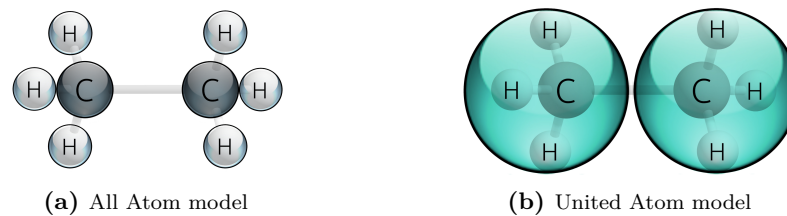
Figure 2.1: Ethane molecule modeled by (a) all atom and (b) united atom approaches.
