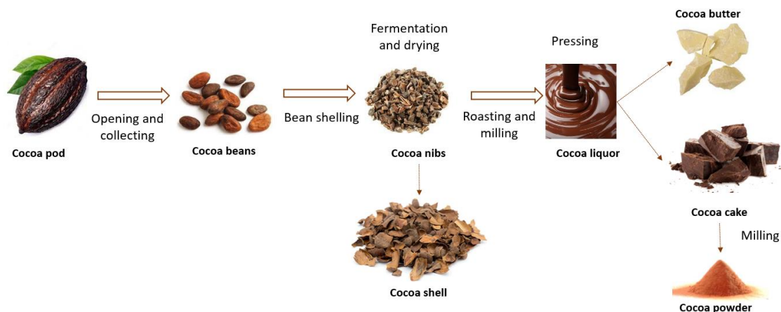
Fig. 1 Summary of the transformation process of cocoa pods into cocoa butter and cocoa powder.
