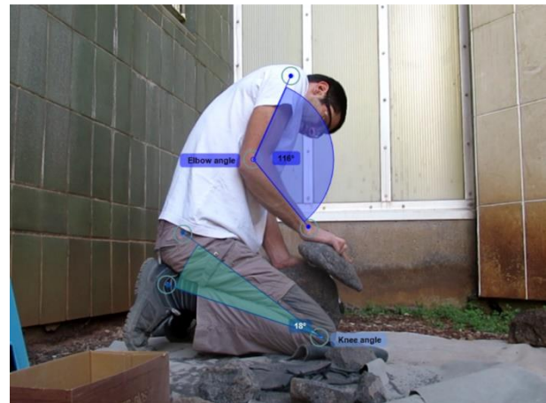
Figure 8: Sample instance for angle measurement of knee flexion and elbow extension using Kinovea software.
