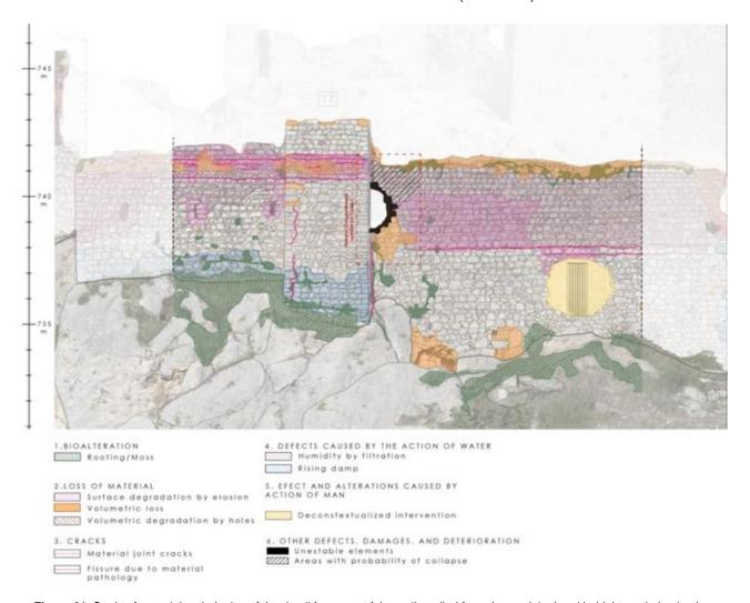
Figure 21: Study of material pathologies of the detail fragment of the wall studied from the model printed in high-resolution by the stereotomy of the construction.
