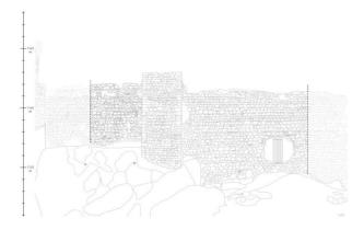
Figure 19: Detailed drawing of each of the elements that make up the chosen wall fragment. First plane for later study of material pathologies.
