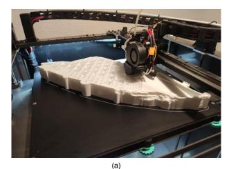
**Figure 12**: Photographs when the first model was being printed in resin with an experimental high-resolution printer: a) View of the lightened grid of the model and b) impression of details.
