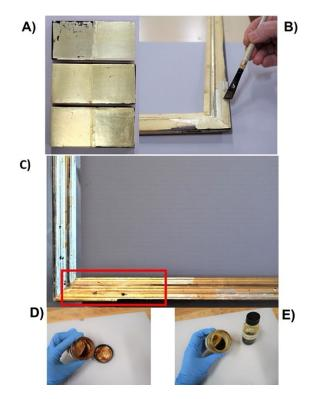
Figure 4 – A) Samples of traditional matte and burnished 13ct gold leaf testing MSA paints. B) Retouching the matte gilded slips with MSA paints. C) Combined approach to retouch burnished passages using MSA with Soluvar Gloss varnish (D) followed by dye/pigment tinted A81 resin glaze (E)
