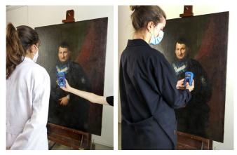
Figure 2 – Sequence of light measurements in front of an artwork characterized by a dark colour palette.
