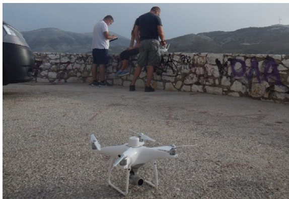
Figure 4. The DJI Phantom 4 RTK UAS at the take-off area.
