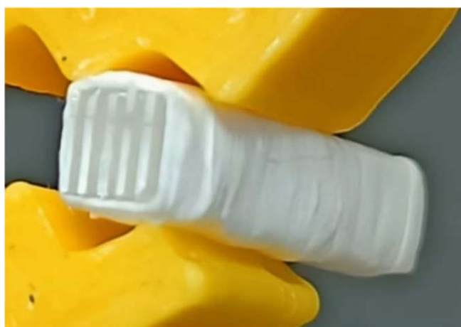
Figure 4. Photo of a 300\ \mu\text{m} BGO- 300\ \mu\text{m} BaF 2 metapixel of total dimensions 3 \times 3 \times 15\ \text{mm}^3 . The difference in color and refractive index between the two materials is directly visible as a change in shade.
