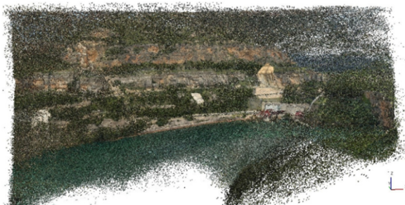
Figure 10. Dense point cloud of the main area.
