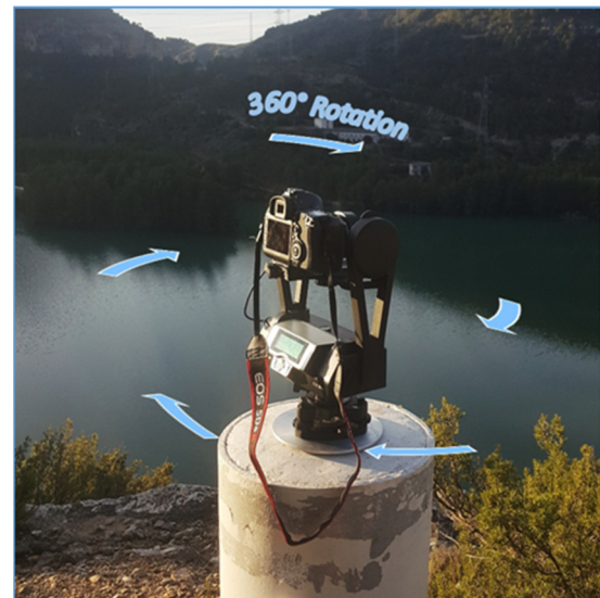
Figure 5. Camera mounted on the Gigapan for acquiring the panoramic images.
