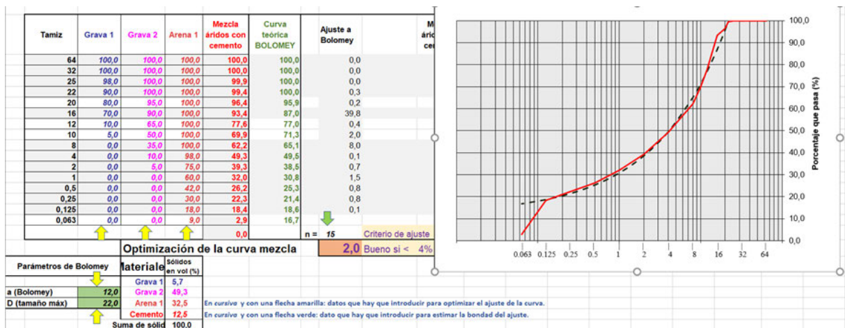
Figure 3. Result of the adjustment of aggregates to the theoretical curve.
