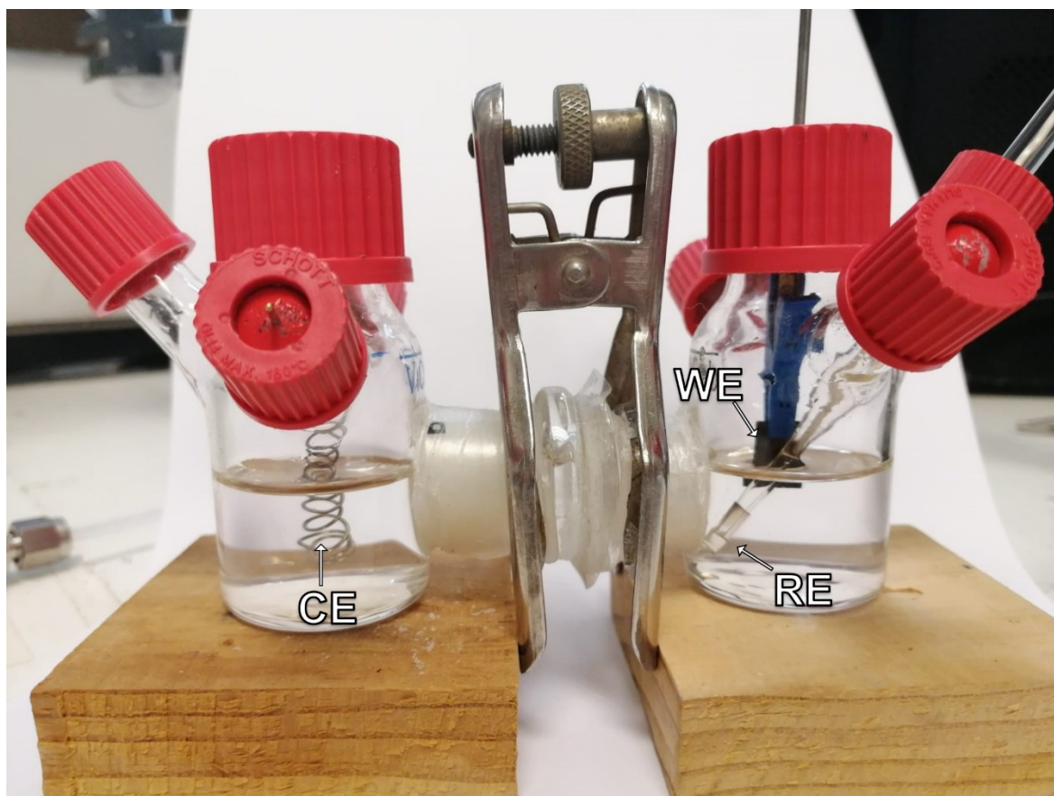
Figure 3 H-Cell Setup with WE, CE and RE
