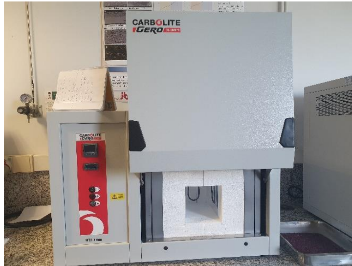
Figure 17: Carbolite Gero high temperature oven used for conventional sintering
