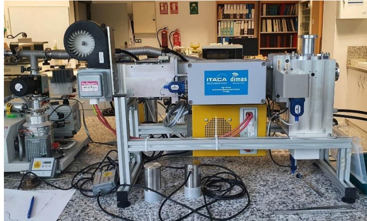
Figure 20: Monomodal microwave oven designed at ITACA-UPV
