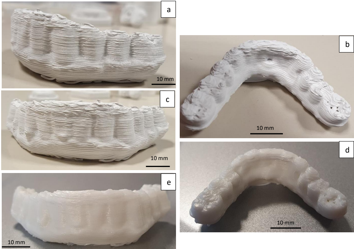
Figure 55: Denture; a) b) c) before sintering; d) e) after sintering
