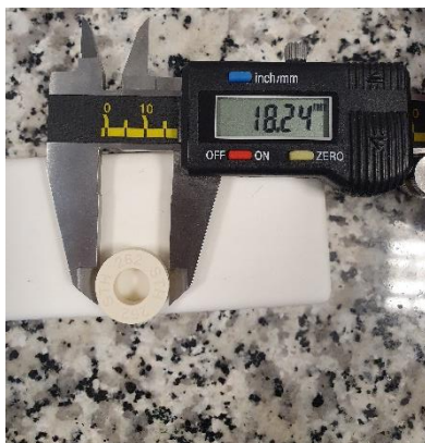
Figure 19: Size PTCR-STH after sintering
