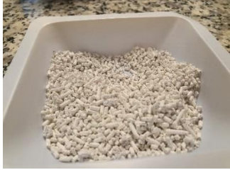
Figure 15: Zirconia ( ZrO_2 ) + binding agent
