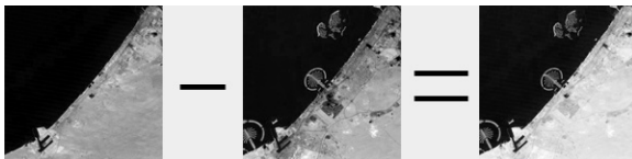
Figure 3. Image Algebra Change Detection: Substraction of pixel-values of two images to identify the differences (FIS, Uni Bonn).
