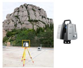
Figure 2. TLS used in the study, Leica ScanStation P50. In the background, the characteristic Montserrat landscape can be appreciated: stepped slopes where vertical conglomerate intercalation of and fine layers of sandstone and siltstone.
