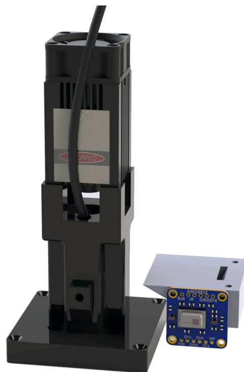
Fig. 5. Laser support and thermographic camera.
