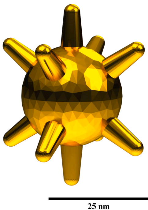
Fig. 10. Nanostar geometry used in the modelization.
