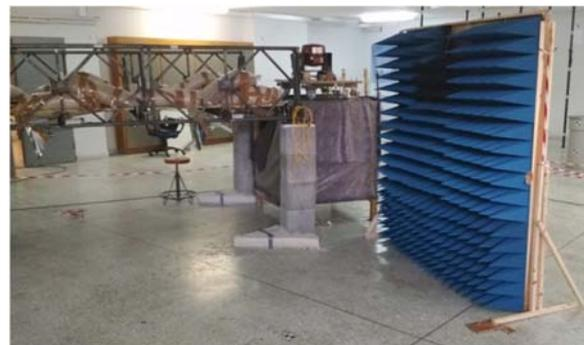
Figure 3. Special barrier surface for the absorption of reflected electromagnetic signals.
