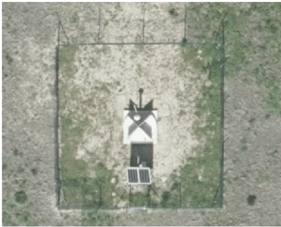
Figure 8. RAG's MSST Stangenmuehle/Fenne, Saarland, LVGL nr. 6707 0 402 00, as to be seen in RAG's orthophoto at 3 cm GSD, aerial flight campaign at noon, April 25 th , 2021. Mapped area 15 m x 14 m. Image courtesy RAG.
