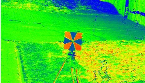
Figure 2. Example landmark target in initial point cloud, computed with GNSS / IMU trajectory.
