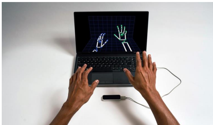
Figura 5. Leap Motion Controller en funcionamiento https://www.ultraleap.com/product/leap-motion-controller/
