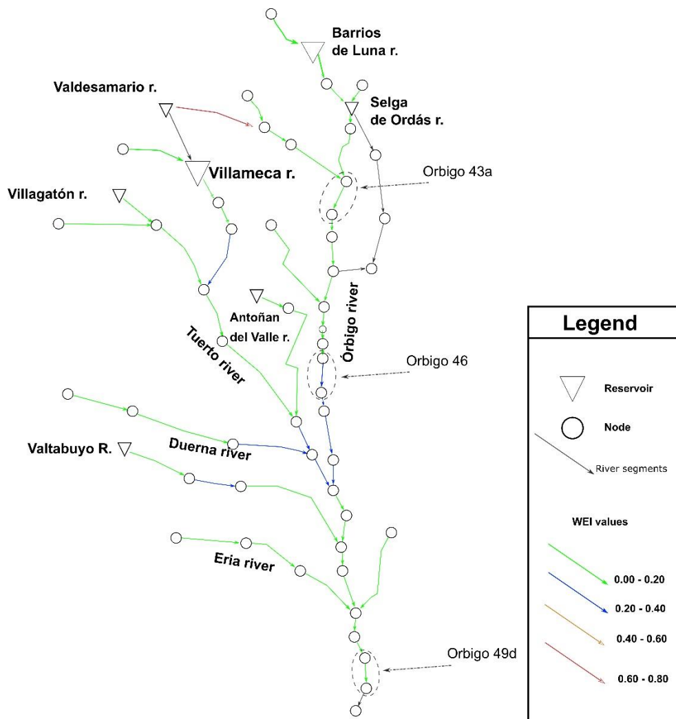
Figure 4. Plan view of the water exploitation index (WEI + ) in each river stretch based on the entire simulated period.
