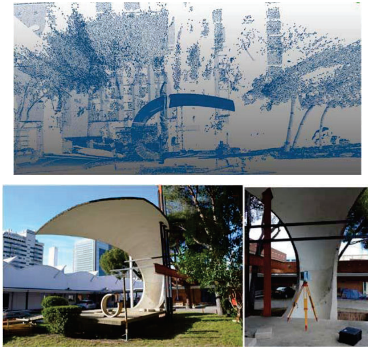
Figure 10. Point cloud of the riblike sheet, stations of scanning.
