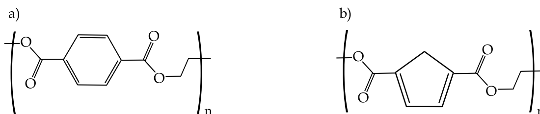
Figure I.1.3.3. Chemical structure of a) petroleum-based poly(ethylene terephthalate) and b) biobased poly(ethylene furanoate) from 2,5-furandicarboxylic acid.
