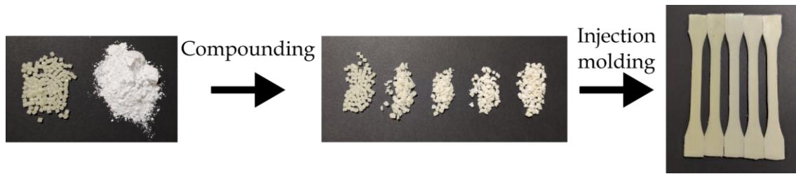
Figure III.2.2.6. Processing steps carried out to prepare the P(3HB- co -3HHx)/nHA parts; from left to right: as-received P(3HB- co -3HHx) pellets and nHA powder, compounded pellets of the nanocomposite, injection-moulded parts.
