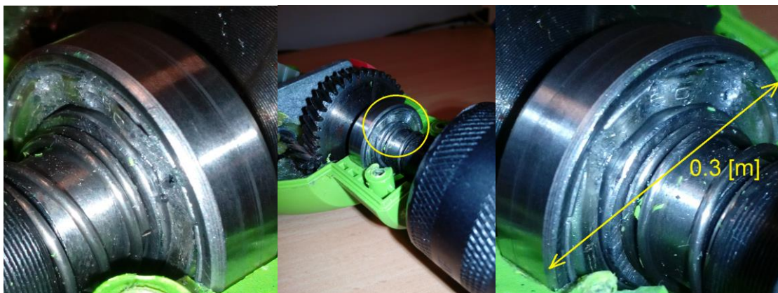
106 Figure 3 EID with damaged front bearing (indicated by yellow circle)
