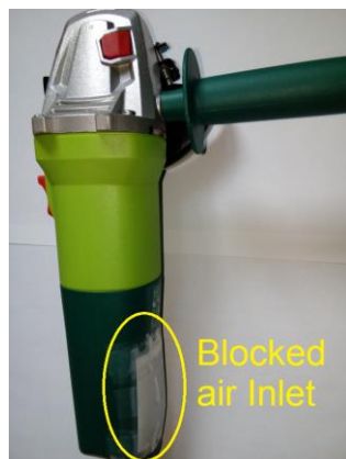
Figure 6. Angle grinder with 1 blocked air inlet
