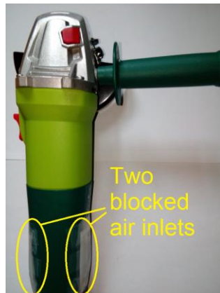
Figure 5. Angle grinder with 2 blocked air inlets
