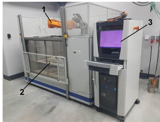
Figure 5. Experimental setup (1—robotic manipulator; 2—immersion bath; 3—control cabinet).
