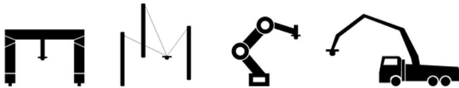
Figure 5.1 Different systems used to obtain large extrusion-based 3D concrete printing machines. a) Gantry, b) cable-suspended, c) robotic arm, d) robotic arm coupled to a modified truck.
