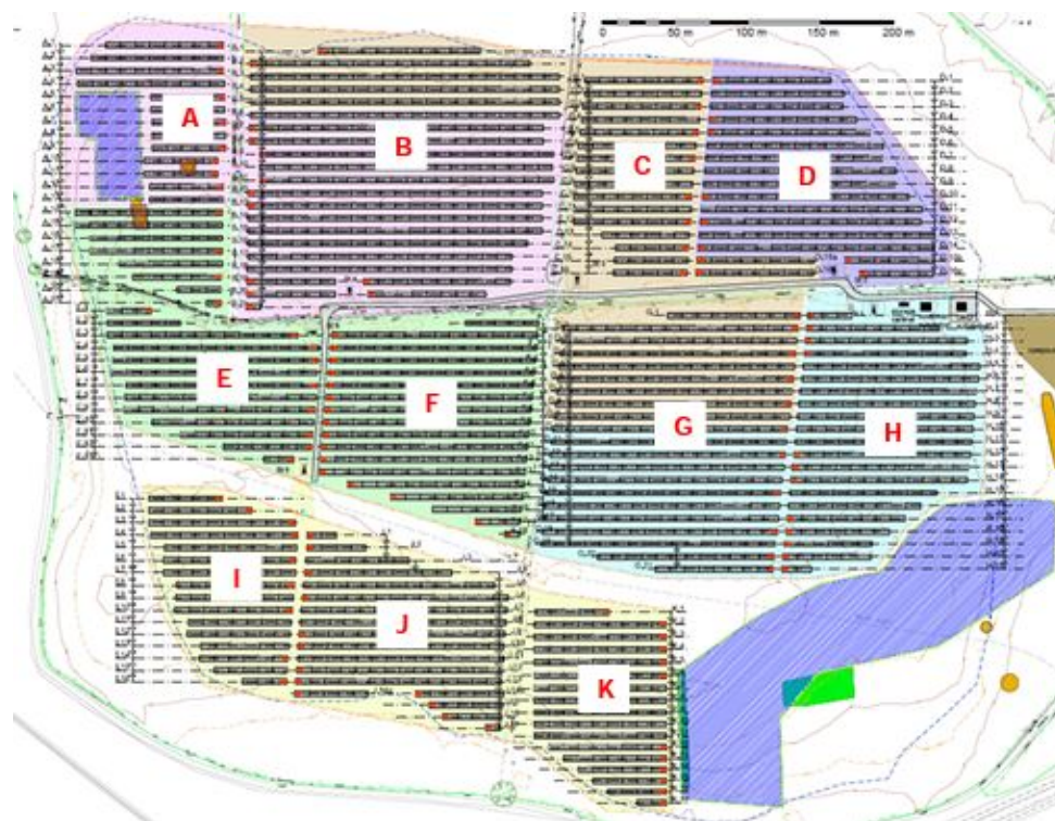
Figure 3.3: System A layout. Each zone corresponds to a central inverter
