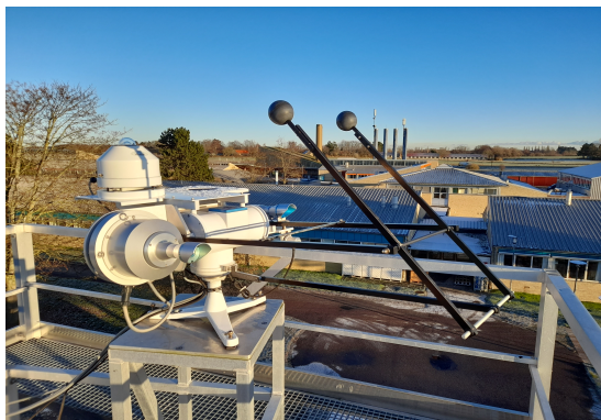
Figure 3.8: DHI pyranometer and DNI pyrhelimeter in System B's weather station
