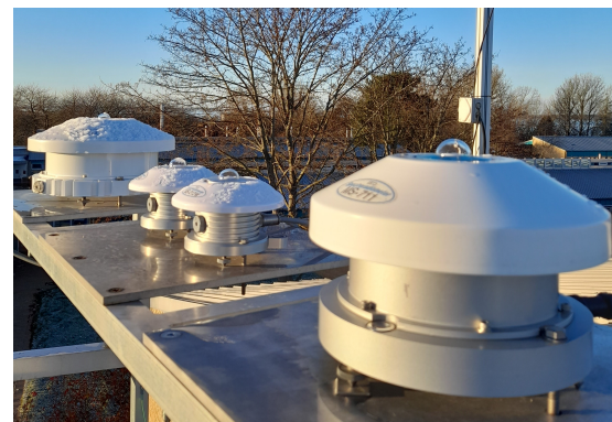
Figure 3.9: Horizontal solar radiation sensors in System B's weather station
