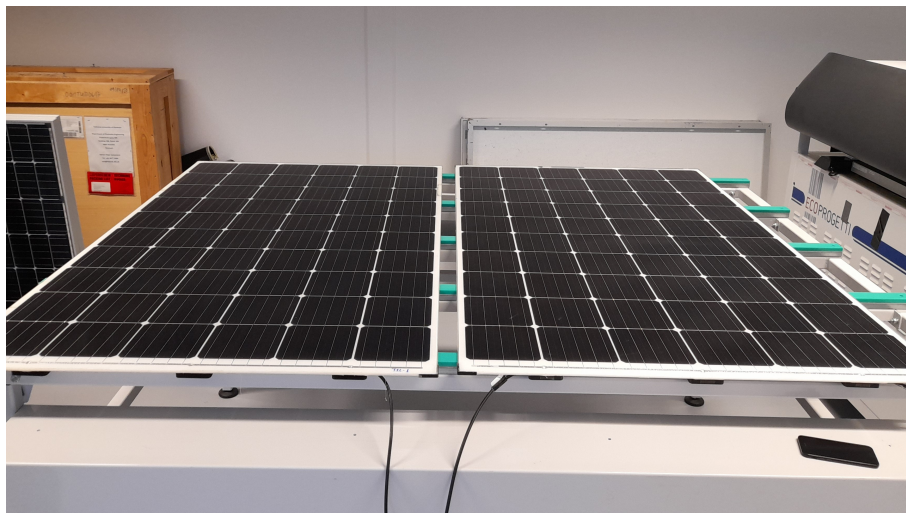
Figure 5.8: Visual inspection of the bifacial module. Left: Fielded module. Right: Reference module
