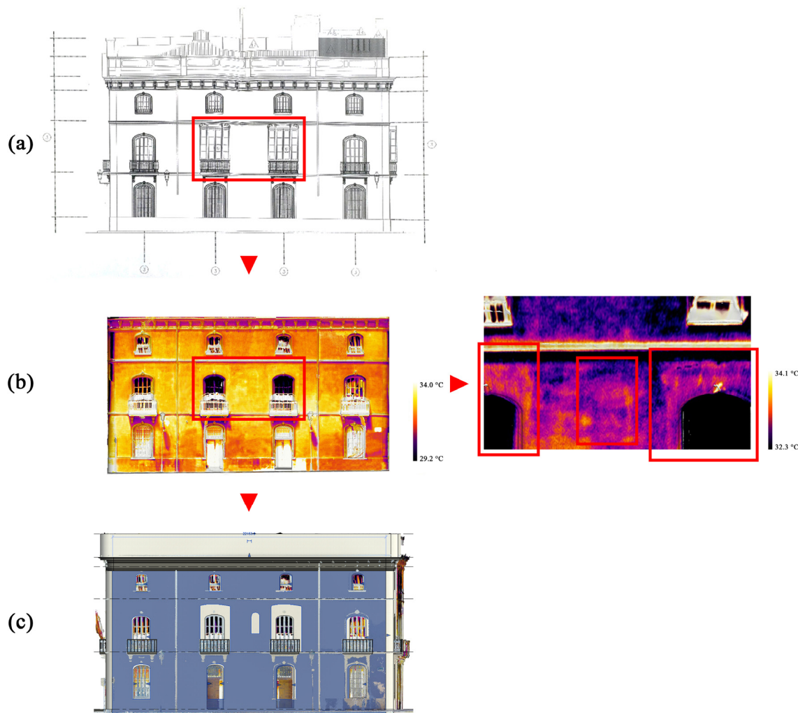
Figure 17. Eastern façade. Superimposition of different data in the HBIM environment: (a) condition mapping from 1995; (b) TIR orthoimagery showing the thermal anomalies (different temperature scales); (c) virtual reconstruction of the “A” and “C” anomalies according to the historical plan and further reconstruction of the central “B” anomaly.
