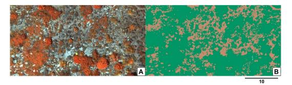
Figure 3. (A) Zenithal view of a section of the Area 1 point cloud in false-colour infrared. (B) Point cloud classified in vegetation (green) and ground (brown) classes.
