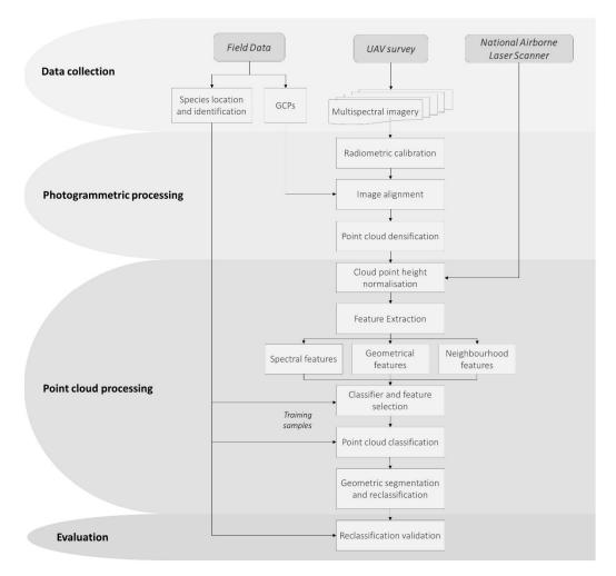
**Figure 2.** Workflow of the proposed methodology. Abbreviations: UAV: unmanned aerial vehicle, GCPs: ground control points.
