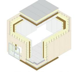
Axonometric exploded view of the module (Cross Laminated Timber)
