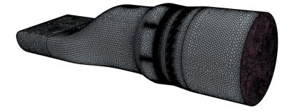
Figure 4. Global external surface reference mesh (75M elements).
