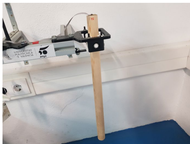
Figure 13. One of the references used to calibrate vertical MOI test stand.
