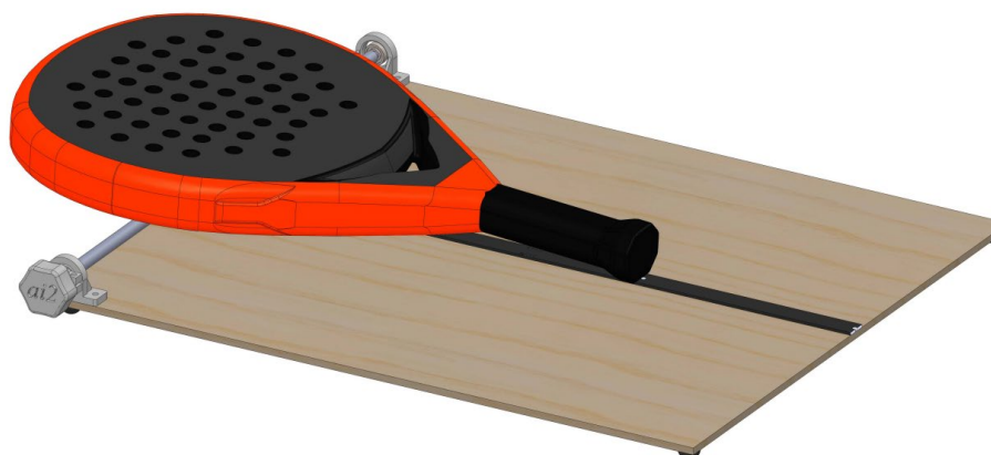
Figure 2. The device used to determine the COM of padel rackets.
