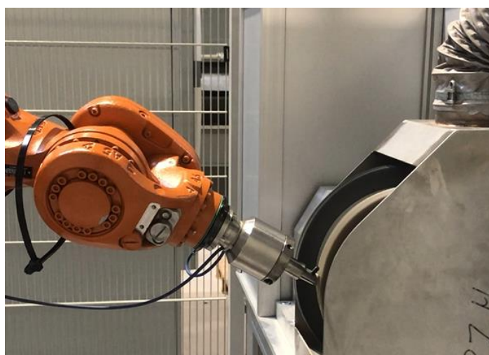
Figure 4.3: Robotic arm used for brushing.
