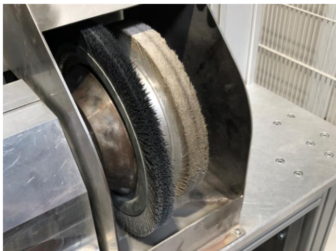
Figure 4.4: Disk brush used for brushing.
