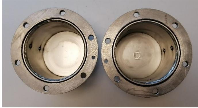
*Figure 2. Radon accumulation containers*
