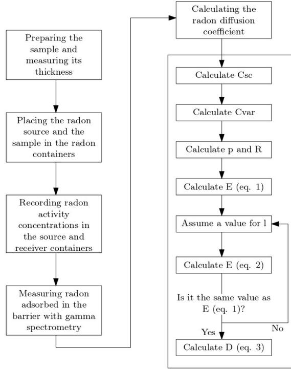
Figure 3. Flow chart of the measurement process and calculation of the radon diffusion coefficient
