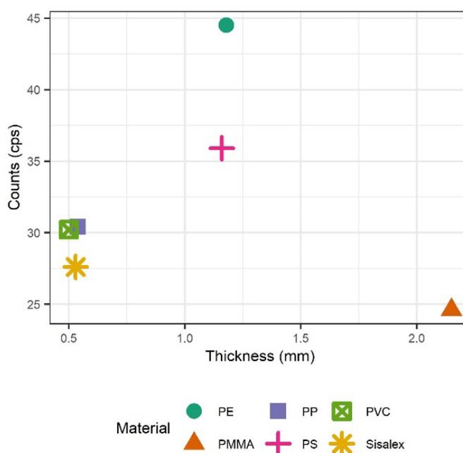
Figure 7. Radon adsorbed by each material compared to its thickness
