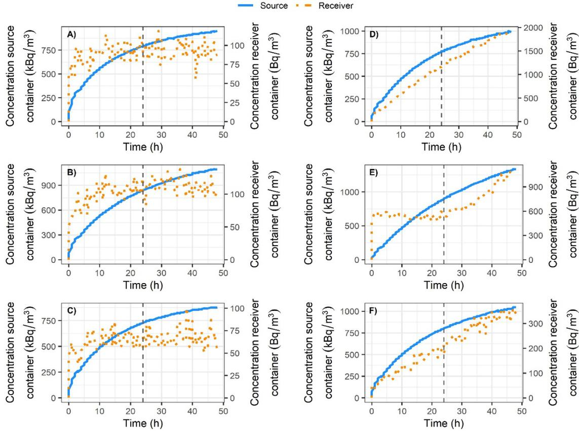
Figure 6. Radon concentration in the source chamber (solid line) and the receiver chamber (dashed line). The materials tested are A) PP, B) PVC, C) PMMA, D) Sisalex, E) LDPE and F) PS
