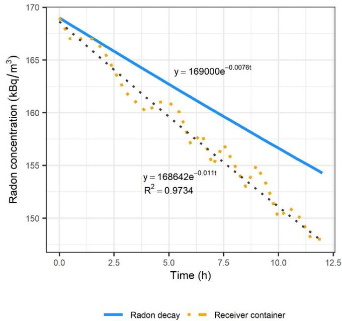
Figure 5. Radon leakage test performed in the receiver container
