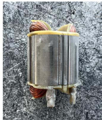
**Figura 5:** Estator o inductor
