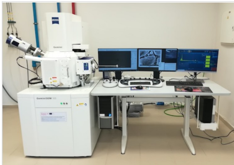
Fig. III.21. Field Emission Scanning Microscope (FESEM) ZEISS ULTRA. (Source: Electron Microscopy Service, UPV).
