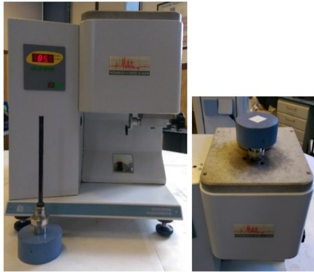
Fig. III.11. The extrusion plastometer for melt flow index (MFI) test.
