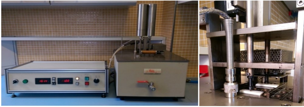
Fig. III.8. The VICAT/HDT equipment and the flat-tipped needles adapter for VICAT test.
