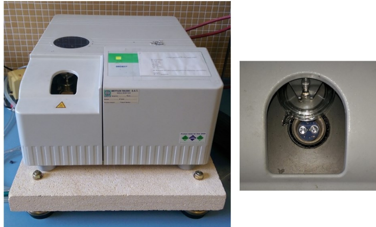
Fig. III.6. The Mettler-Toledo-821 DSC and sample holder images.
