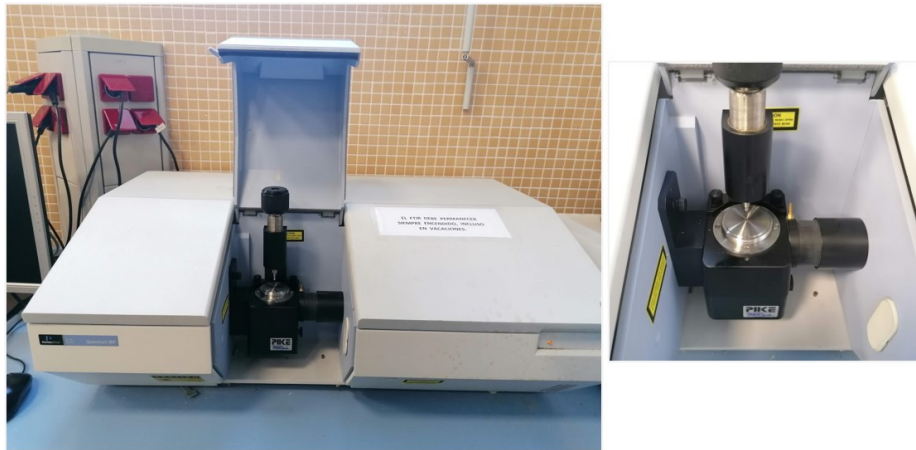
Fig. III.20. A JASCO 615 plus spectrometer equipment and the ATR tools.
