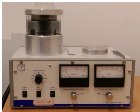
Fig. III.22. Sputter Coater equipment Emitech SC7620.
