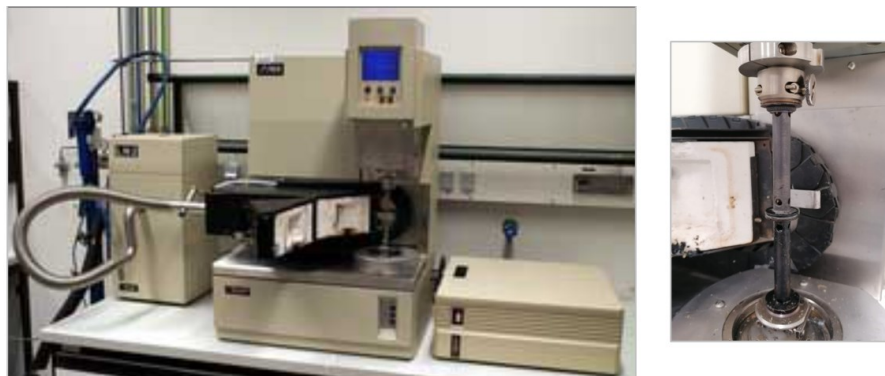
Fig. III.10. The Ares N2 rotational rheometer (adapted from Forschungszentrum Jülich, GmbH) and the parallel plates geometry.
