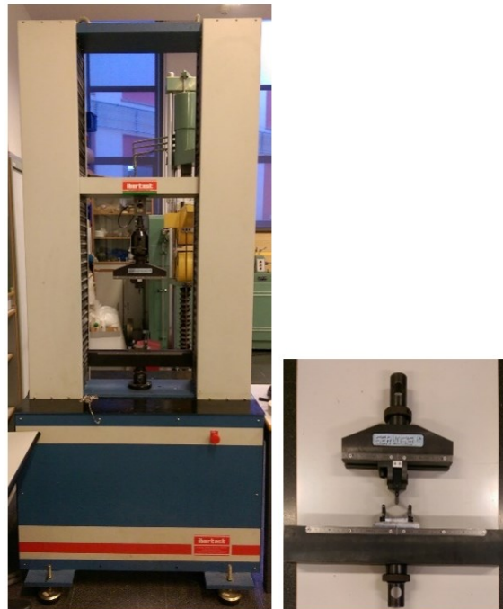
Fig. III.16. IBERTEST electromechanical universal testing machine and adaptable clamp for flexural test.
