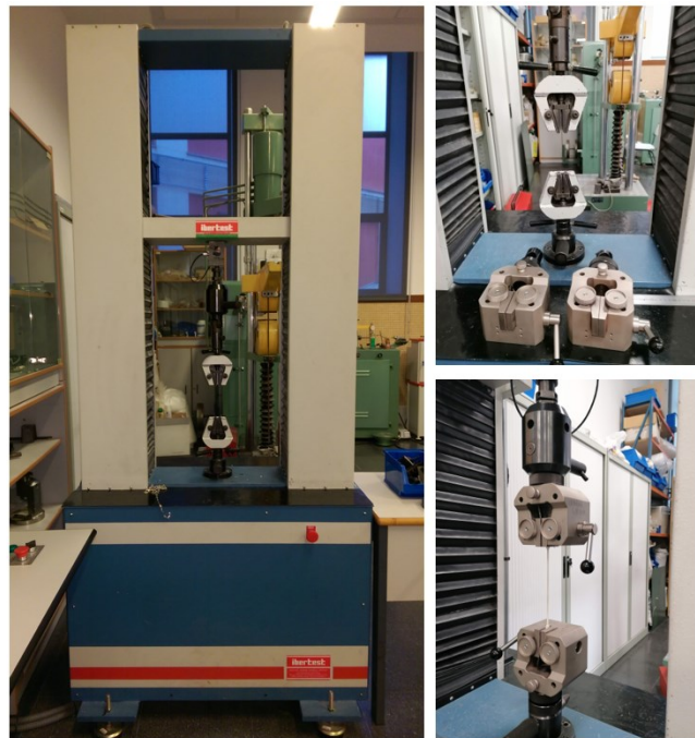
Fig. III.13. IBERTEST electromechanical universal testing machine and adaptable clamp for tensile test.
