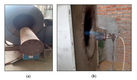
**Figure 8.** This figure shows the exhaust fan and types of gas burners handcrafted (**a**) 3-nozzle gas burner; (**b**) 2-nozzle gas burner.
