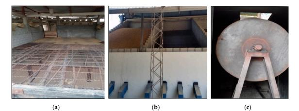
**Figure 7.** The figure shows (**a**) a dryer of a rectangular type chamber made with bricks and metal pipes; (**b**) a multichamber dryer made with perforated plates, bricks, and type C metal beams, (**c**) Gas rotary dryer, used for aging rice.
