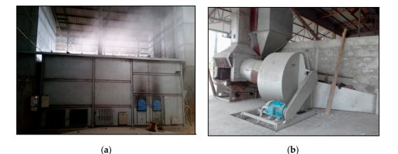
**Figure 10.** Shows two types of biomass dryers. (**a**) Double chamber dryer; on the left is the drying chamber and on the right is the combustion chamber. Brazilian technology, first-generation processing plant; (**b**) Handcrafted dryer with a drying chamber, combustion oven, ducts, and an exhaust fan in a second-generation processing plant.
