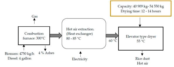
Figure 13. Temperature and dry time, using biomass. First category processing plant.
