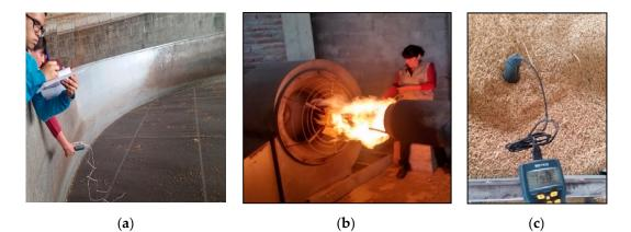
**Figure 6.** This figure shows (**a**) measurement of the drying chamber using a temperature recorder with type K thermocouples; (**b**) measurement of the inlet hot air temperature by the extractor, a ceramic-coated lance thermocouple; (**c**) measurement of the initial and final humidity of the product, spear type grain moisture meter.
