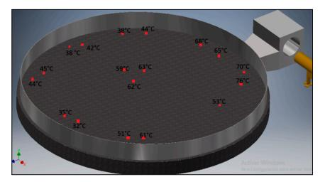
Figure 15. Chamber temperature. The capacity of 400 quintals (18,200 kg).
