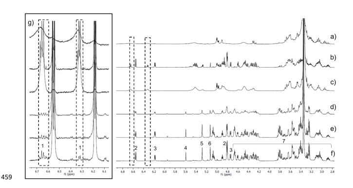
**Figure 1.** <sup>1</sup>H NMR spectra of pure adulterants and pure honeys in DMSO-d6: a) rice syrup, b) corn syrup, c) barley syrup, d) citrus pure honey, e) sunflower pure honey and f) heather pure honey. g) magnification from 6.0 to 6.8 ppm. Main resonances of monosaccharides are identified as follows: 1 β-maltose, 2 β-glucopyranose, 3 α-glucopyranose, 4 α-fructofuranose, 5 β-fructofuranose, 6 β-fructopyranose, 7 aliphatic protons and other oligosaccharides.
