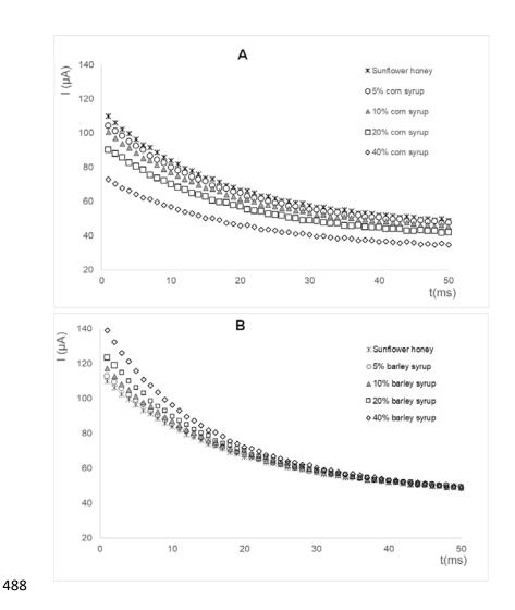
**Figure 5.** Variation of the current intensity as a function of time for a potential step (400 mV with gold electrode) by adding different levels of barley syrup (Figure 5.A) or corn syrup (Fig 5.B) on the sunflower honey.
