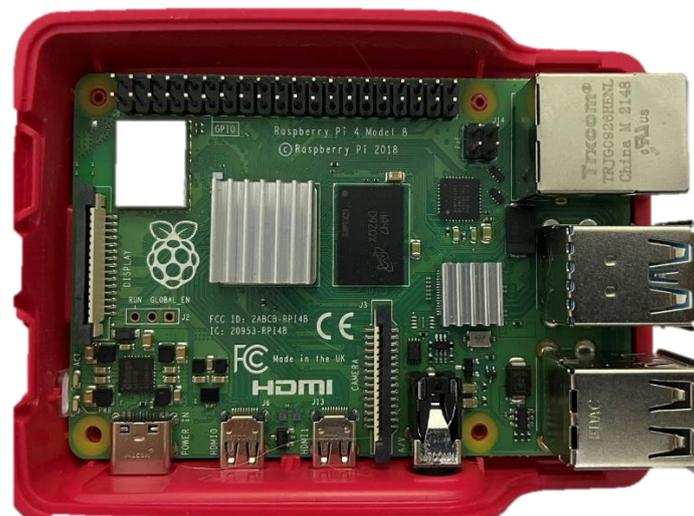
Figura 16. Raspberry Pi 4 model B
