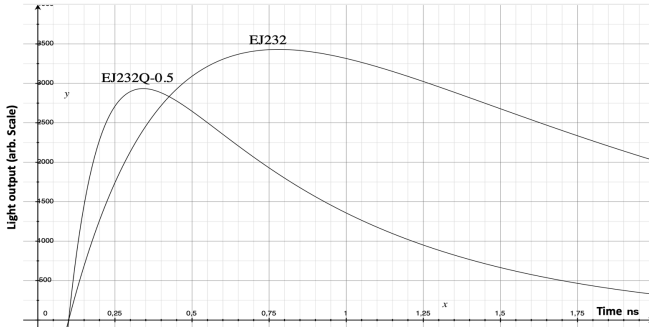
Fig. 9: Pulse shape of EJ232 and EJ232Q-0.5 plastic scintillators (from Eljen technologies data sheets)
