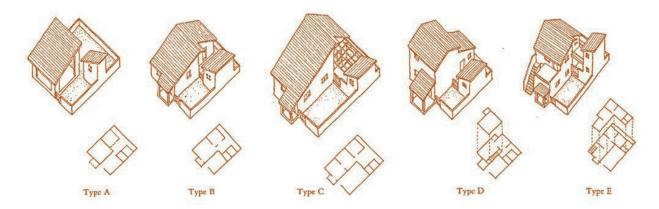
Figure 6 |: Unit plans of Incremental Housing, Navi Mumbai (Correa, 2020).
