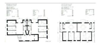
Figure 6 | "Minimum income" housing prototypes established by the OHS for blocks in line, half-rise houses and houses with 2 and 3 bedrooms.
