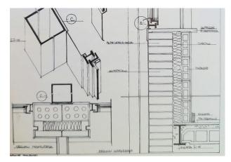
Figure 10 | Detail of the nasturtium wall with insulation in the air chamber. Architect: Francisco de Asís Cabrero Torres-Quevedo. 1961. (Climent Ortiz, X. (ed). "Francisco Cabrero, arquitecto").
