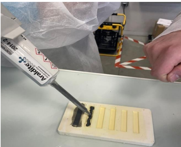
Figure 17: Manufacturing of the 2014-2 epoxy samples at the lab
