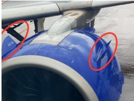
Figure 47: Location of the devices on the engine nacelle Figure 46: Typical appearance of the Strake
