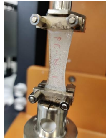
Figure 45: Bubbles inside PC-N-1
