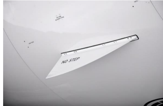
Figure 47: Location of the devices on the engine nacelle Figure 46: Typical appearance of the Strake
