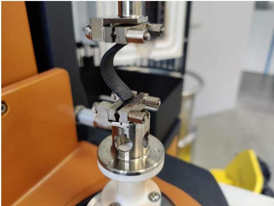
Figure 39: Embrittlement causes the EPOXY-N-1 sample to break during tests
