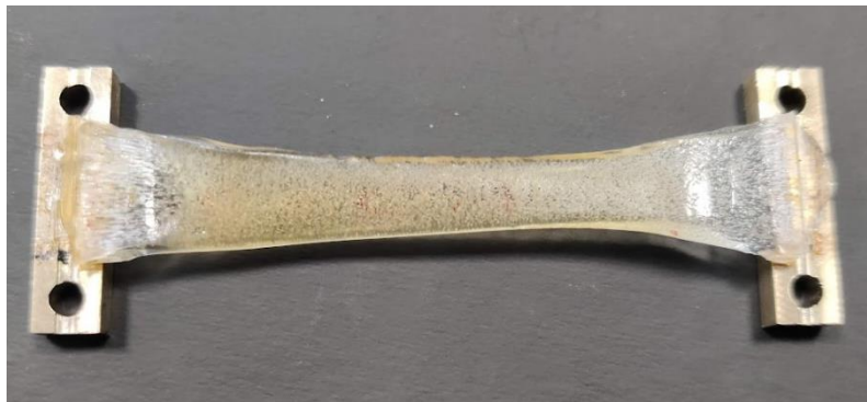
Figure 44: Bubbles inside PS-HC-1 sample
