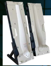
Wind turbine blade mold. 1700 x 520 x 330 mm. *Printed by BTU (Brandenburg University of Technology Cottbus-Senftenberg).
