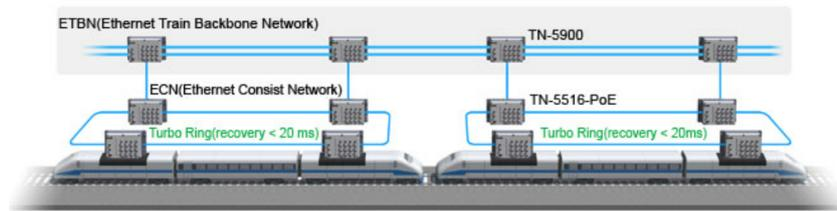
**Figure 3.1: Ethernet ring in rail vehicles [37]**
