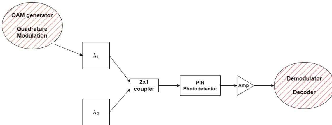
**Figure 3.3: System overview using Optisystem**
