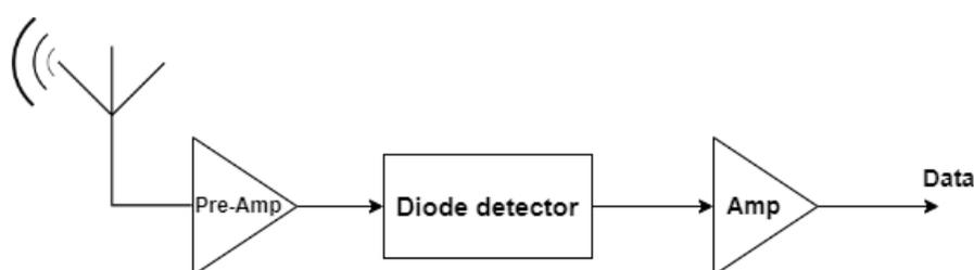
**Figure 2.15: Receiver block diagram**
