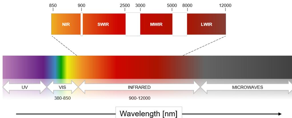
Figure 2.2: Infrared band [14]
