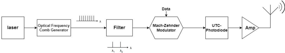
**Figure 2.18: Simple scheme for photonic generation of THz signals using comb generator**
