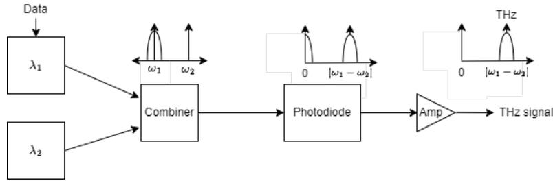
**Figure 2.6: Simple scheme for photonic generation of THz signals using two lasers**
