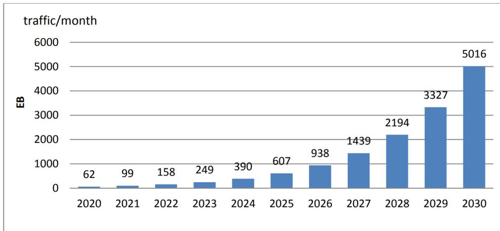
**Figure 1.2: Estimation of global mobile traffic between 2020 and 2030 [6]**
