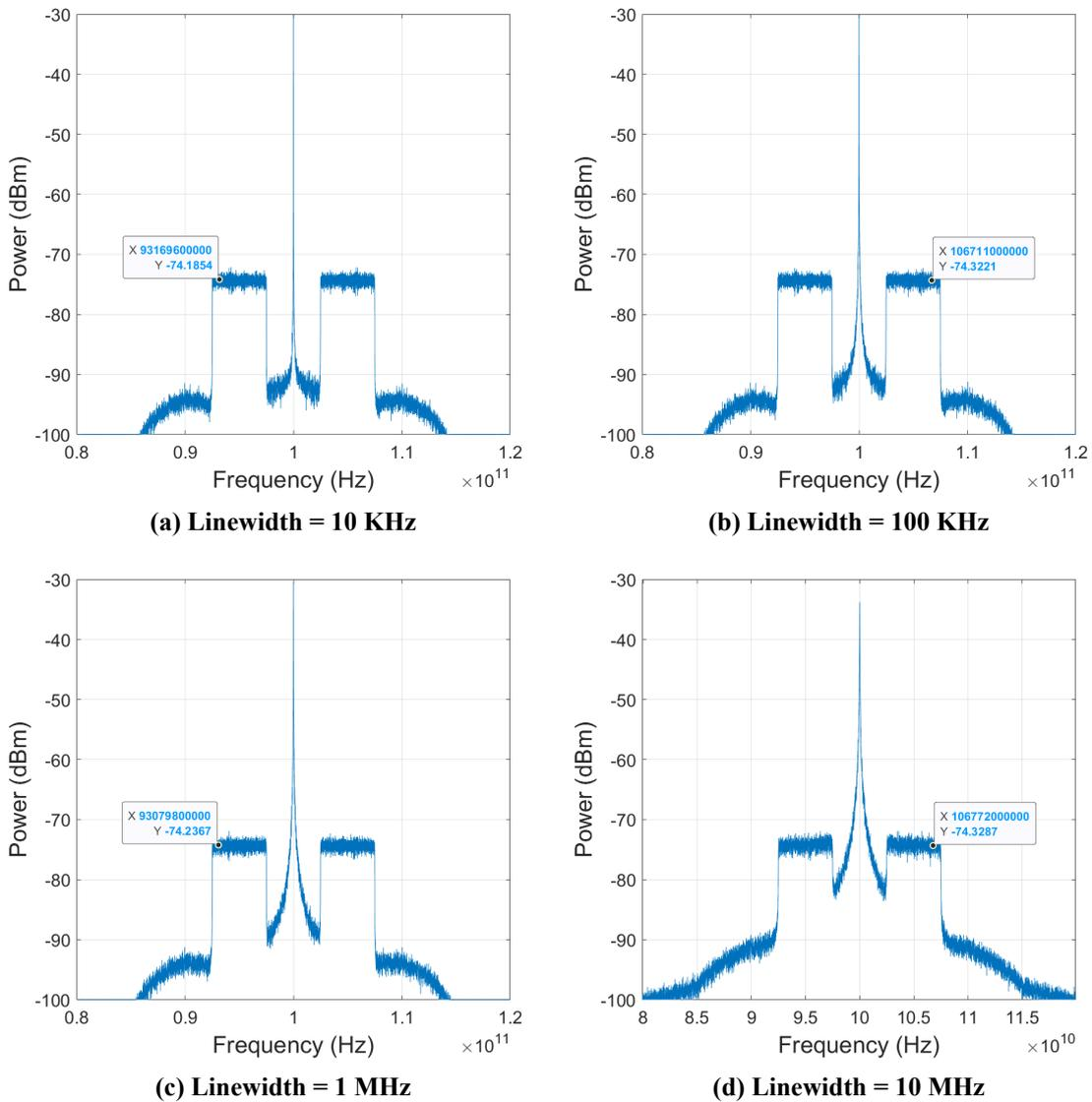
**Figure 3.18: RF spectrum after photodiode for 5.299 dBm output power, 100 GHz frequency and different linewidth values**
