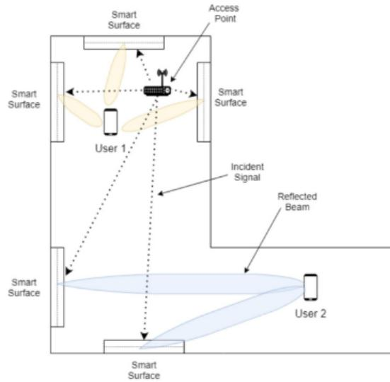
**Figure 2.20: Smart surfaces system [36]**
