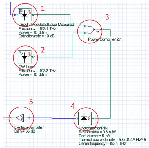
**Figure 3.6: Scheme overview using Optisystem**
