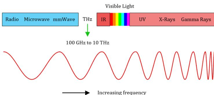
**Figure 2.1: Radio spectrum [12]**
