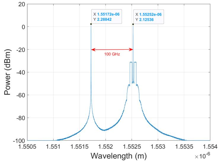
**Figure 3.13: Optical Spectrum after combination of both Lasers**
