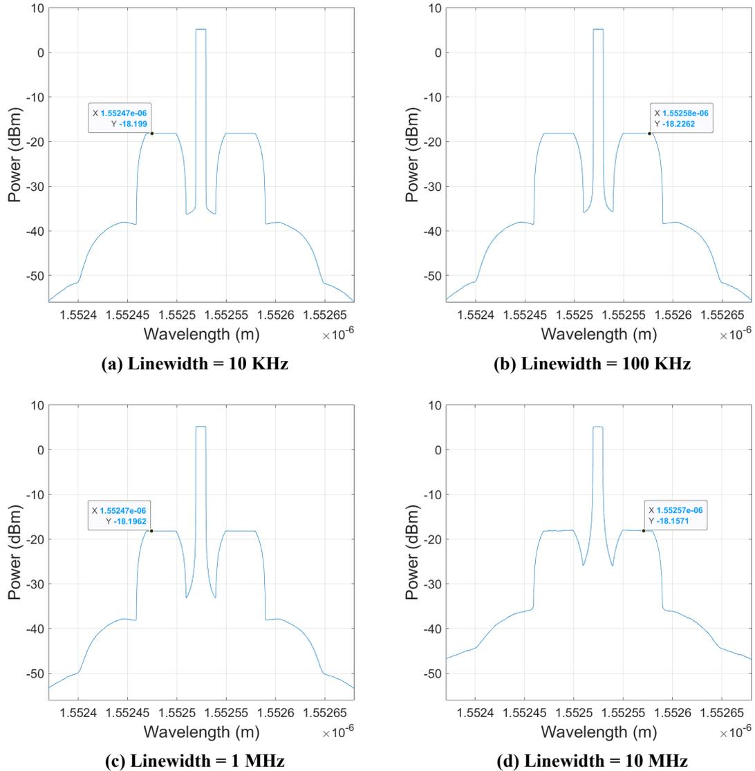
**Figure 3.17: Optical spectrum after the fixed laser for 5.299 dBm output power, 100 GHz frequency and different linewidth values**
