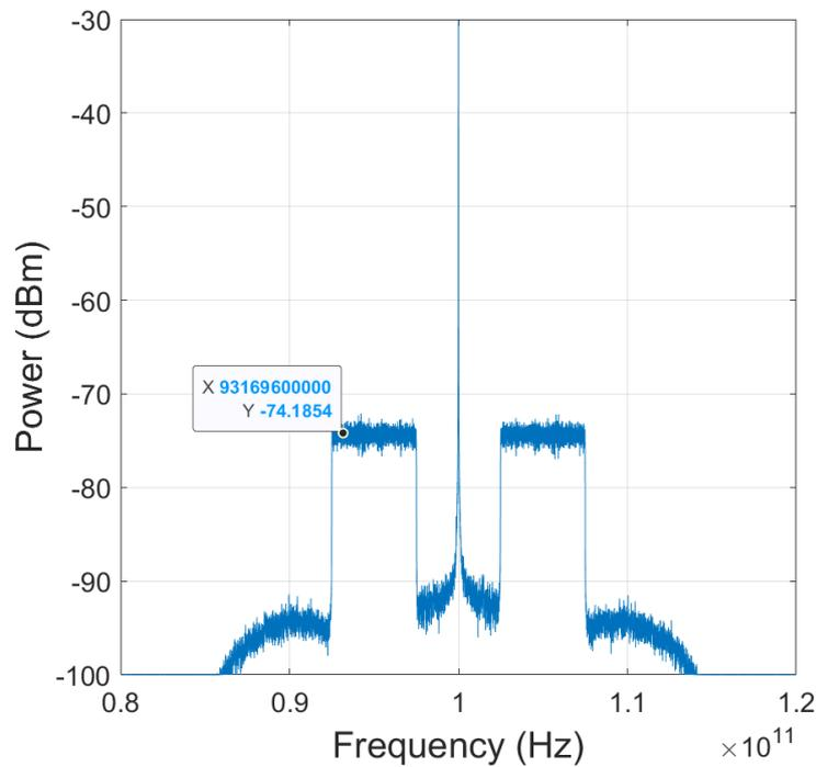
**Figure 3.14: RF Spectrum after Photodiode**
