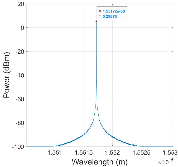
**Figure 3.12: Optical Spectrum emitted by variable laser**
