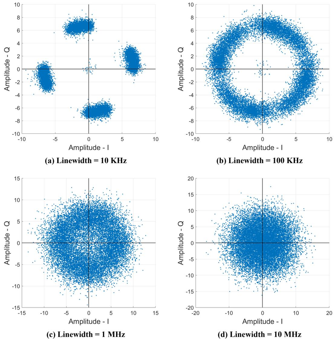
**Figure 3.16: Output constellation for 5.299 dBm output power, 100 GHz frequency and different linewidth values**
