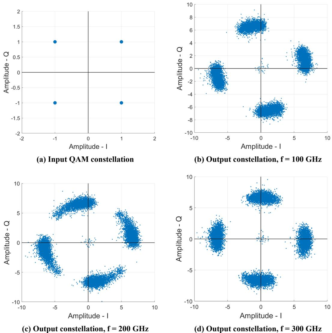
**Figure 3.8: Output constellation for 5.299 dBm output power value for different frequencies**
