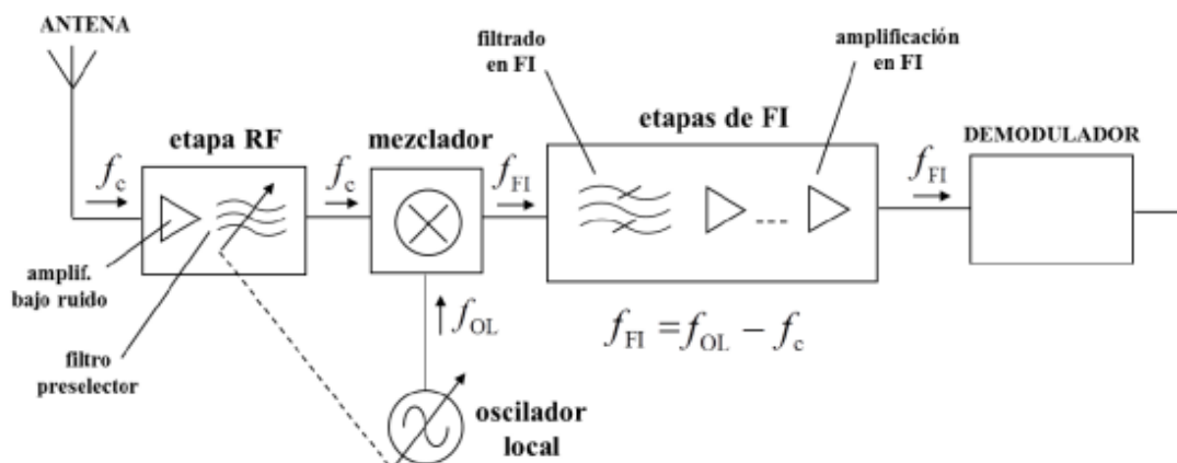
Diagrama 2. Receptor Superheterodino.
