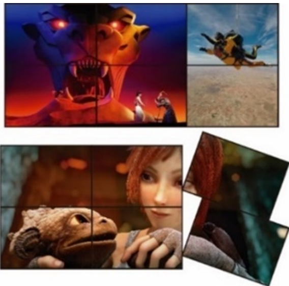
Figure 1. 2-section mosaic (top) and 1-section warp (bottom) examples of videowall display distributions
