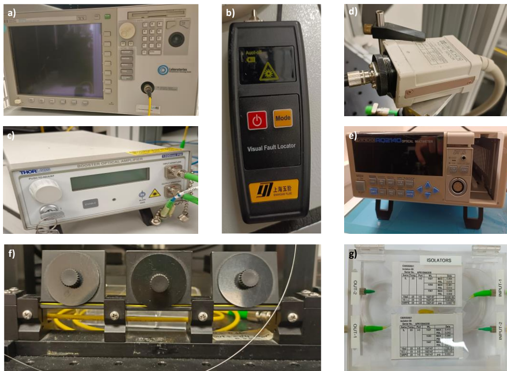
Figure 13. a) Optical Signal Analyzer. b) Visual Fault Locator (red laser). c) Booster Optical Amplifier. d) Power meter cap. e) Power meter. f) Polarizer. g) Isolator
