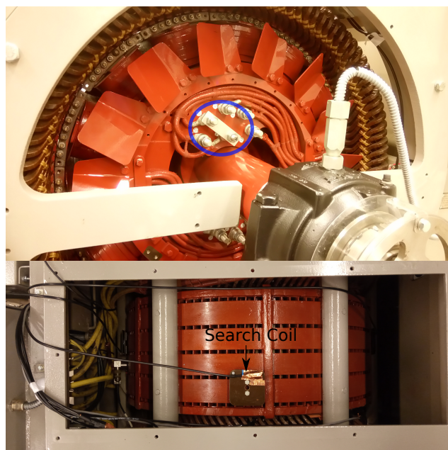
Fig. 2. The location of the shorted turns tap on the rotor (top) and the location of the stray magnetic field sensor installed on the stator back side of a SPSG.
