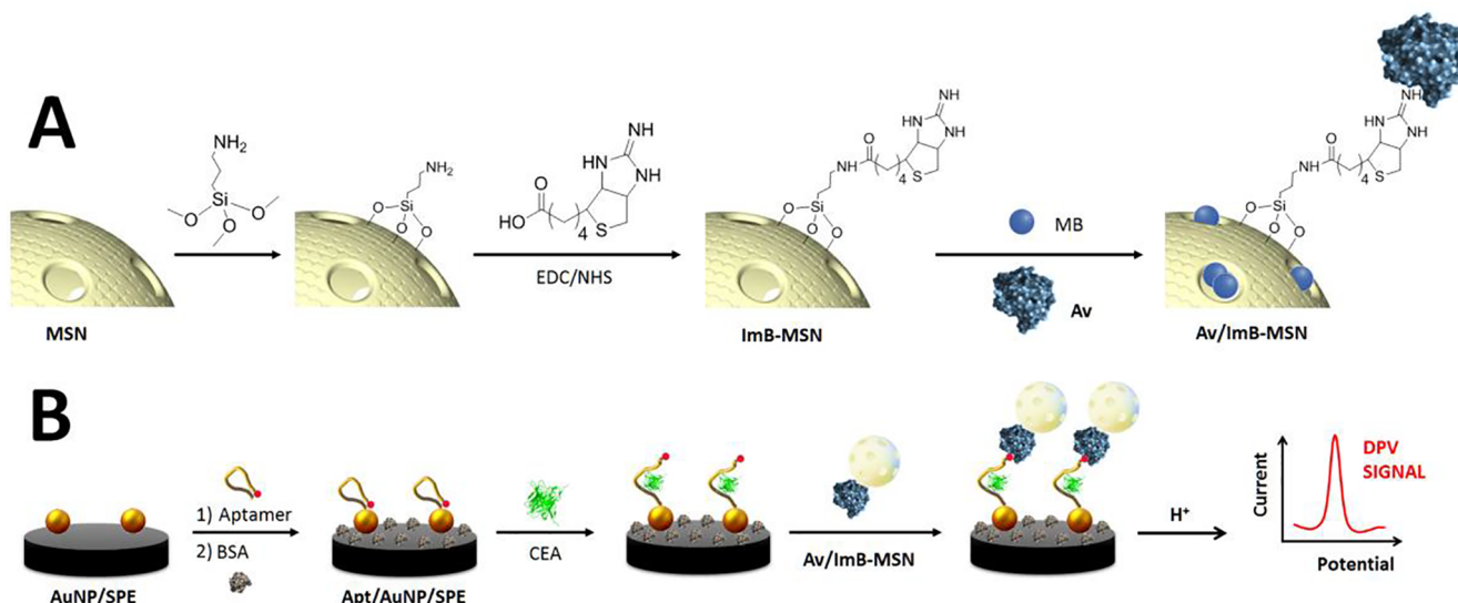
Fig. 1. Schematic display of the processes involved in the preparation of the Av/ImB-MSN nanocarrier (A) and the construction and use of the aptasensor for CEA determination (B).
